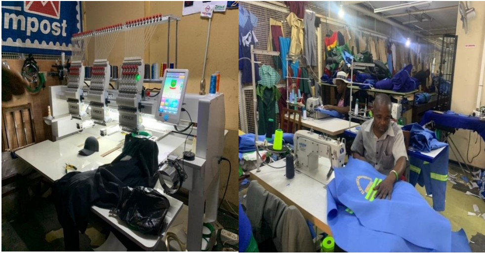
The new state of the art Embroidery Machine at the Zimpost Production Unit.
